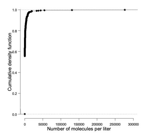
Supplementary Figure S1. Plot of the cumulative probability density of the eDNA concentrations to obtain the threshold for detection. The 95% percentile was 8,221 molecules per liter (i.e. x-value with y-value 0.95 in this figure) indicating that CT-values higher than 45 cycles are likely to be caused by double-stranded non-target DNA.
